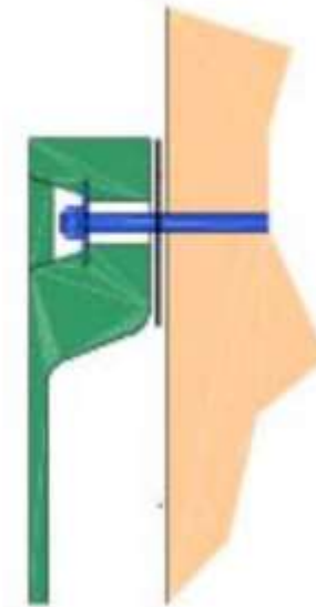
Figure 4.3 - Example of Face Fixing
